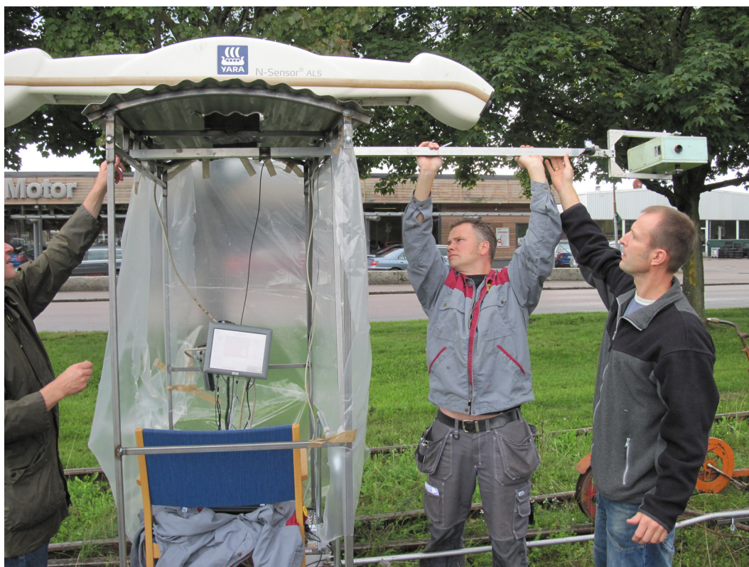
Figure 1. The test rig. A N-sensor is mounted on top of a small wagon pulled by a inspection trolley. The software of the sensor includes information on biomass and position.
